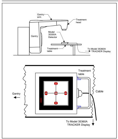
Figure 2-4. Setup for 0-Degree Gantry Angle (NOTE: Build-up not shown for clarity)
